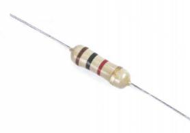
The colour bands on this resistor indicate that it has a nominal value of 1000 ohms
