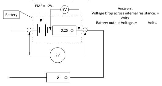
**2.** Determine the value of the internal resistance?.
