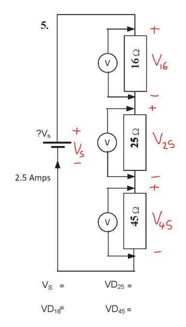
What is the total voltage drop across the resistors (i.e.  $V_S$ ) in the circuit at right?
