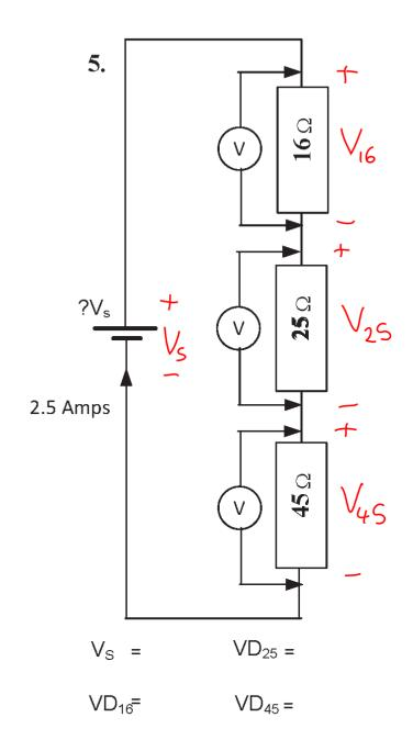
What is the total voltage drop across the resistors (i.e.  $V_s$ ) in the circuit at right?
