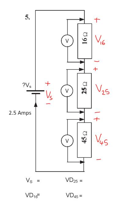
For resistors, the series formula derived from KVL using Ohm's Law:
